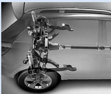
Rear suspension includes automatic self-levelling.
