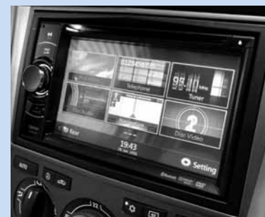
NX501E satellite navigation system, showing touch-screen display.
