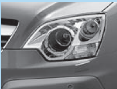
Xenon headlights with high-pressure washers.
