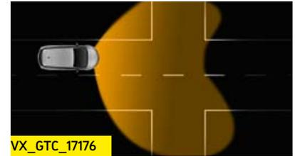
**Pedestrian area light.** Wider spread of light (an extra eight degrees left and right) illuminates potential hazards (up to 20mph).
