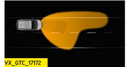
**Adverse weather light.** Wiper or rain sensor activated for better vision in bad weather conditions (up to 45mph).
