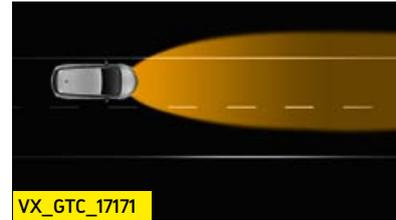
**High beam with assist.** Automatically switches from high to low beam as it detects oncoming or proceeding vehicles (over 25mph).
