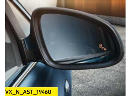
**Side Blind Spot Alert.** Available as part of the optional Perimeter Protection Pack on Sport and SRi models, this ultrasonic-based system helps prevent a potential collision with a vehicle in the neighbouring lane by continuously screening the blind spots on both sides of the car and provides a visible warning if the indicator is set to change to a lane where another car is detected.
