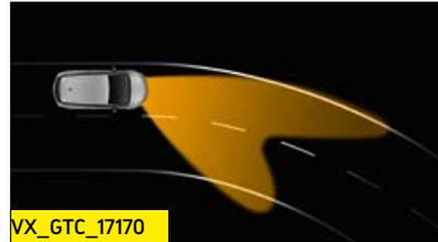
**Dynamic curve light.** Activated by steering angle and speed, the headlights swivel up to 15 degrees into the curve (any speed).
