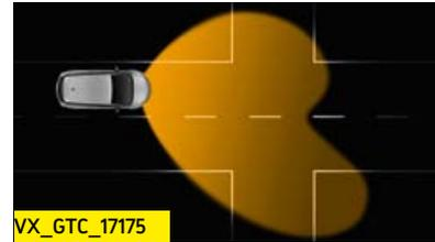
**Town light.** Wider and lower spread of light. Activated by vehicle speed together with street lighting (20-35mph).
