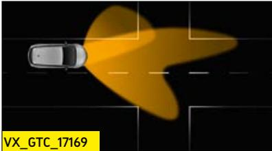
**Static cornering light.** Throws light 90 degrees left or right for enhanced lateral vision (up to 25mph, also when reversing).
