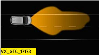
**Motorway light.** 140 metre range, higher and brighter than normal low beam, without dazzle (over 60mph).
