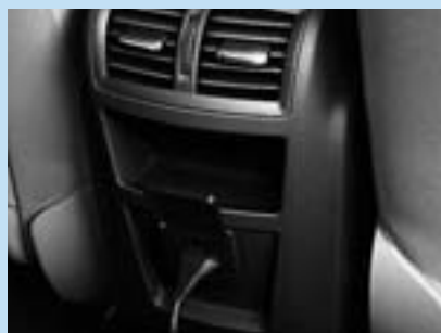
230-volt rear power outlet.
