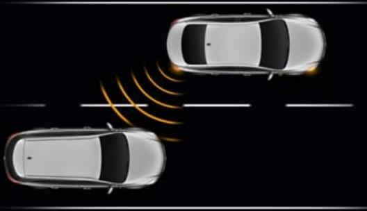
**Side blind spot alert.** This system helps prevent a potential collision with a vehicle in the lane either side of the car by continuously monitoring both blind spots. If a vehicle enters one of those blind spots, a warning light flashes in the relevant door mirror. If you indicate to change lanes, a warning sound alerts you to the potential danger.
