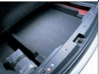
Underfloor storage. Choose the optional 15-inch steel spare wheel and Meriva's luggage compartment also features an underfloor storage area with three compartments including a special one designed for a warning triangle (not supplied).
