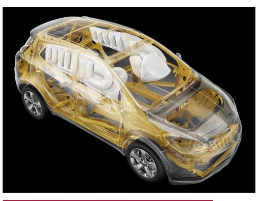
**The Mokka's passive safety systems are uncompromising and comprehensive.** It's difficult to imagine how you could be better protected inside your Mokka. You are surrounded by a high-strength steel rigid passenger cell as well as front, side and full-length curtain airbags. On the outside, pedestrians are protected by bumpers that use low-density foam, designed to reduce the risk of leg injuries should the unthinkable happen.
