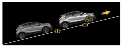
**Hill Start Assist (HSA).** HSA will stop you rolling back unintentionally on steep hills, by automatically releasing the brake at just the right moment when pulling away on a gradient.
