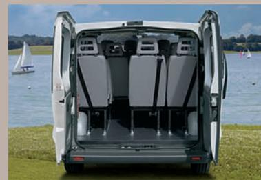
**'Quiklok'.** Fourth-row seats are mounted on aluminium rails with 'Quiklok' quick-release fittings.
