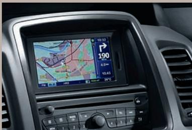
**Satellite navigation.** Optional TomTom-based system features a useful fascia mounted/hand-held remote control unit.
