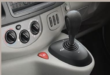
**Tecshift.** Combines the main features and flexibility of automatic transmission with the performance and control of a manual gearbox.
