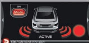
**Side Blind Zone Alert System.** For vehicles fitted with the optional Side Blind Zone Alert system, you can choose to turn it on or off.
