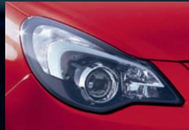
**Adaptive Forward Lighting (AFL).** Optional on New Corsa VXR, the lighting system swivels the beams up to 15 degrees for improved vision as you turn a corner. On Insignia VXR, the standard Intelligent AFL bi-xenon headlights automatically adjust to suit the driving conditions.
