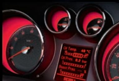
**VXR instruments.** Insignia VXR takes care of driver information via a well-appointed cluster of red accented instruments, with digital graphic display of oil temperature, oil pressure and boost pressure figures.
