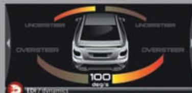
**Dynamics.** Understand your vehicle's behaviour with an understeer and oversteer display.
