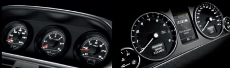
**Sports instrumentation.** The New VXR8 GTS sports instrumentation also features auxiliary gauges that display oil temperature, oil pressure and battery voltage. Vital information easily identified in the sight-line on top of the dash. Ergonomics that put the New VXR8 GTS driver instinctively in control.
