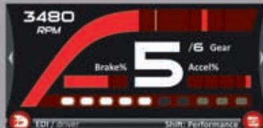
**Driver.** Driver screen keeps you close to key inputs such as RPM, accelerator and brake pedal positions, and gear position.
