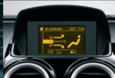
**Electronic Climate Control (ECC).** This allows you to select the temperature to the nearest degree and maintain it regardless of the outside temperature. The system, on some models, can even compensate for the effects of sunlight falling on one side of the car.
