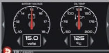
**Gauges.** Select your gauges for real-time information such as Power, Torque, Manifold Pressure, Fuel, Elevation, or Air Temp. (intake or external).
