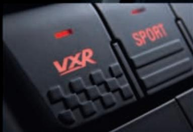
**FlexRide® (Adaptive Stability Technology).** The Insignia VXR FlexRide® provides three different driving modes: select 'VXR' for ultimate driving dynamics or 'Sport' for everyday sporty driving. 'Normal' is the default mode. In extreme situations, FlexRide® automatically adjusts the damping to provide maximum safety and control in every driving mode.
