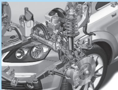
MacPherson strut front suspension.
