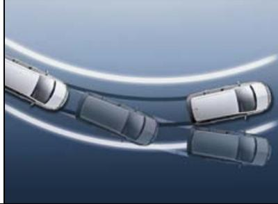
◀ **ESP-plus.** Especially useful on wet roundabouts and greasy roads or whenever a slippery surface catches you out, Electronic Stability Programme-plus (ESP-plus), senses if the car starts to slide on a bend and applies corrective braking to the appropriate wheels to help you regain control.
