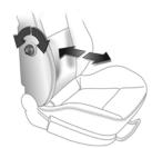
Lumbar support Turn handwheel. Do not lean on backrest when adjusting.
