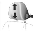
Head restraint adjustment: Press the release button, adjust height and engage.
