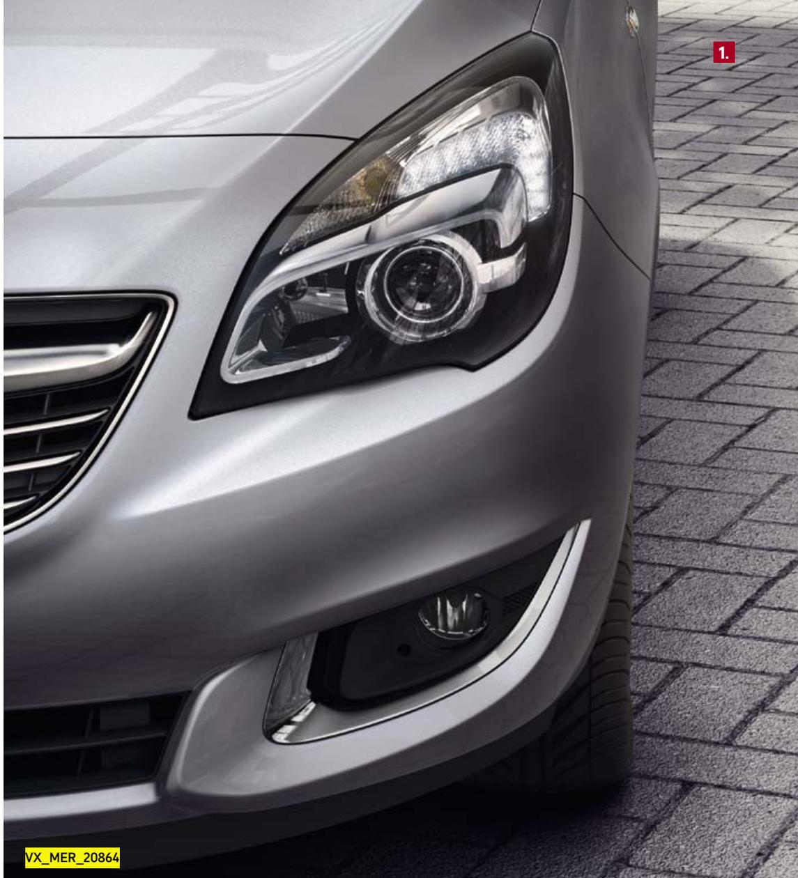
**1. Adaptive Forward Lighting.** This option makes cornering at night safer with dynamic curve light that actually angles your headlights into the bend you're entering. While the static cornering light throws light up to 90° to the left or right so you can see better at low speed corners and junctions.
