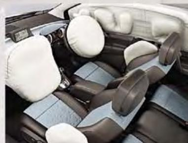
**Airbags.** Meriva is equipped with front and side-impact airbags for driver and front passenger (front only on Expression models). The front passenger airbag can be deactivated for child seat use. Curtain airbags are also standard on Exclusiv, Tech Line and SE models.
