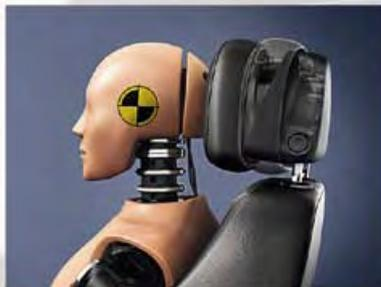
**Active-safety front seat head restraints.** Meriva's active front seat head restraints move up and forward under a rear impact to minimise the risk of whiplash injury and guard against other head and upper body injuries. Standard on Exclusiv, Tech Line and SE models, optional as part of the Protection Pack on Expression, S and Energy.
