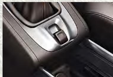
**Electric parking brake.** The electric parking brake not only saves space, it also releases automatically when you drive off, making hill starts much easier.
