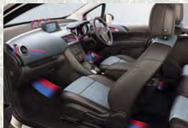
**Electronic Climate Control (ECC).** This optional dual-zone system incorporates air conditioning with a particle filter.
