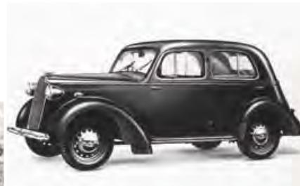
1937 – The Vauxhall 10' H-type, the first British car to have integral construction.
