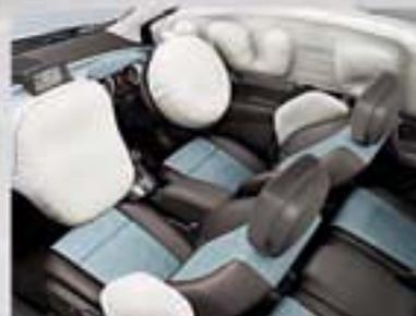
**Airbags.** New Meriva is equipped with front and side-impact airbags for driver and front passenger (front only on Expression models). The front passenger airbag can be deactivated for child seat use. Curtain airbags are also standard on Exclusiv and SE models.
