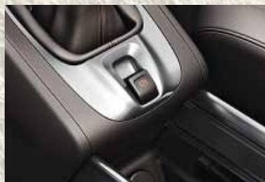
**Electric parking brake.** The electric parking brake not only saves space, it also releases automatically when you drive off, making hill starts much easier.
