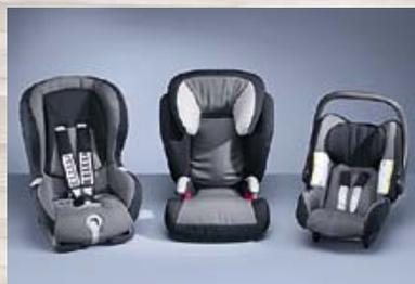
**Child seats.** The rear-facing Baby-Safe (right - up to 13kg) and KID (centre - 15-36kg) seats are fixed with a standard lap and diagonal seatbelt. The DUO ISOFIX (9-18kg - left) can also be attached using the ISOFIX child seat restraint fittings (complete with Top Tether), standard on the outer rear seats of Meriva models.
