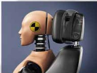
**Active-safety front seat head restraints.** Meriva's active front seat head restraints move up and forward under a rear impact to minimise the risk of whiplash injury and guard against other head and upper body injuries. Standard on Exclusiv, Tech Line and SE models, optional as part of the Protection Pack on Expression, S and Active.
