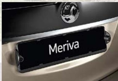
**Rear parking distance sensors.** Activated automatically as you select reverse, this clever system beeps faster the closer you get to an obstruction, rising to a continuous tone at 300mm away.
