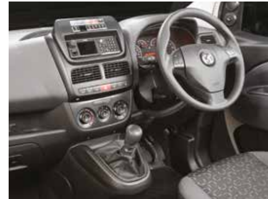
Image shown includes combined 10-way switch panel and aperture for communications head unit.
