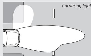
The 'Cornering light' uses an additional bulb and reflector to project a beam of light approximately 90° to the direction of travel when required – for example when turning at junctions or even negotiating tight roundabouts.
